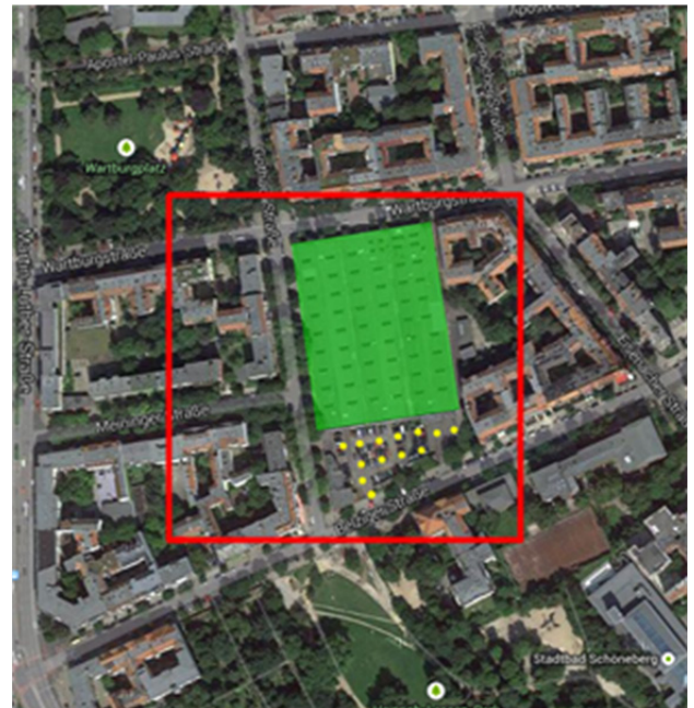
Fig. 1 Simulation area in Berlin-Schöneberg (Google Earth, 2014). Inside the red square 2 m x 2m horizontal grid resolution and outside 8 m x 8 m. The green area in the middle shows the position of the green roof as measure number one and the yellow dots the 13 trees as measure number two.
