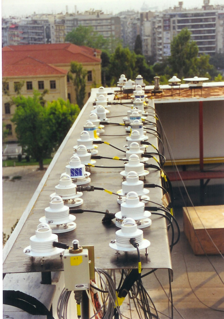
Figure 1: View of the broadband radiometers and spectrometers that took part in the COST/LAP/WMO intercomparison in Thessaloniki, Greece, in 1999.
