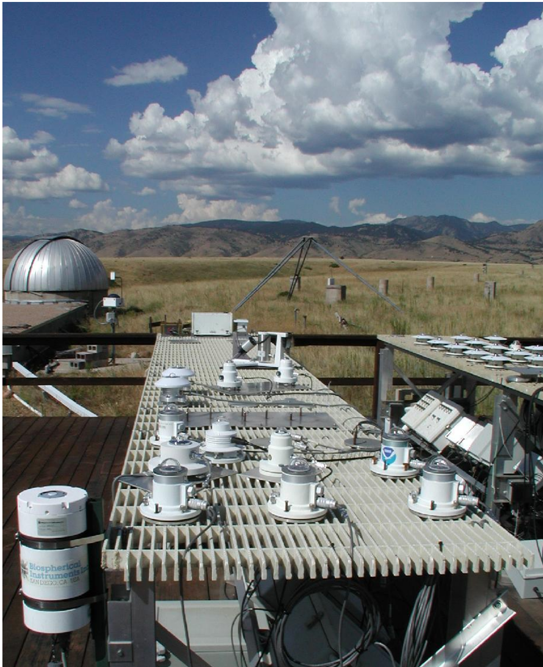
Figure 2: View of 12 UV broadband radiometers at the Central UV Calibration Facility (CUCF), Boulder, CO, USA. These include 4 YES UVB1, 1 older design and 2 newer design EKO, 1 Scintec, 2 Kipp & Zonen, and 1 Solar Light.
