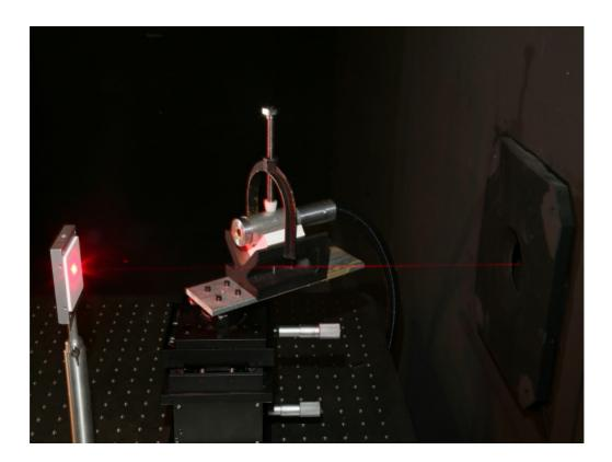
Figure 2 - Alignment of diffuser plate (left) with a HeNe Laser for a laboratory calibration of an array instrument measuring spectral radiance
