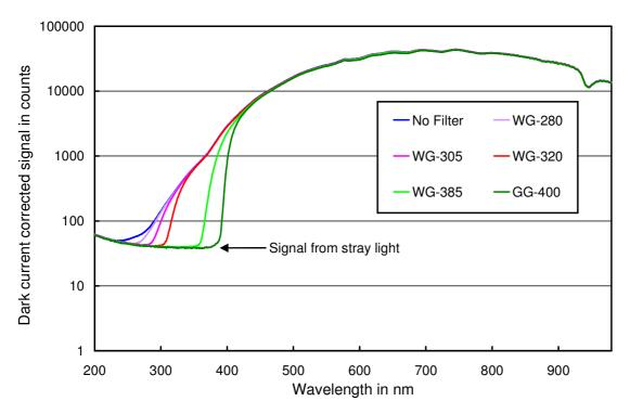
Figure 3 - An example of stray light determination from a spectrograph using cut-off filters
