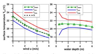
Figure 6: Sensitivity of water surface temperature for variation of wind forcing and depth of the water body.
