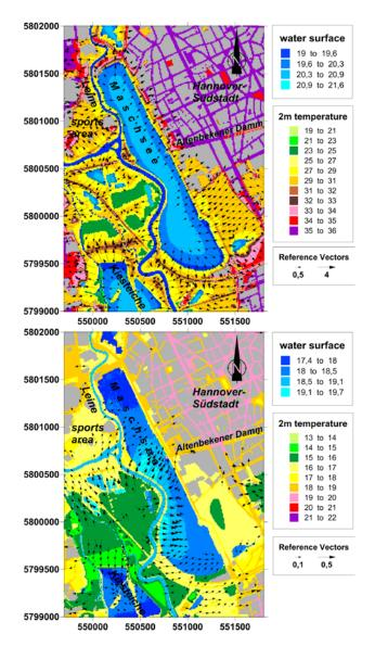
Figure 7: Simulated wind and temperature in 2m a.g. for daytime (above) and for night time (below). ① and ② indicate location of the observation sites.
