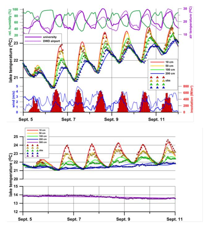
Figure 4: Above: Observed and simulated water temperatures for the centre of the Maschsee (location **0** in Figure 7). Meteorological data are given in the upper and lower panel.
